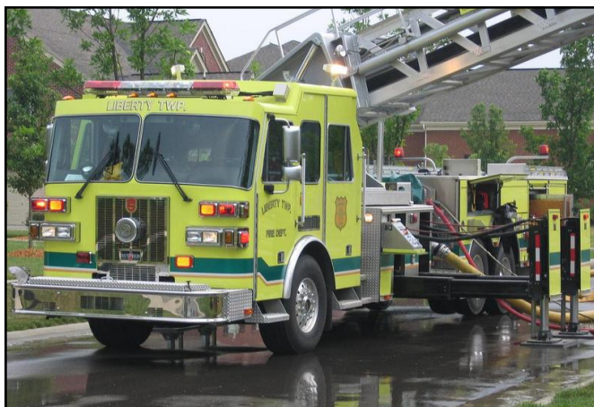
110' Aerial Platform Ladder Truck—purchased in 2004— in action
